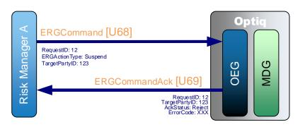
Risk Manager A sends a private **ERGCommand** (U68) message to suspend a trader or an algorithm using a short code, without providing the Firm ID.
