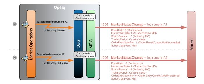
Contract A is in a Continuous trading phase as defined in the **TimeTable** and by the pattern associated to this contract. Instruments A1 and A2 are part of the contract.
